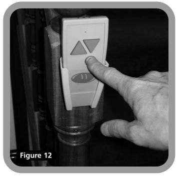
At this time the seat will beep three times whilst the hinge track automatically folds open itself. When the hinge is fully open the stairlift will continue to the bottom of the stairs.
