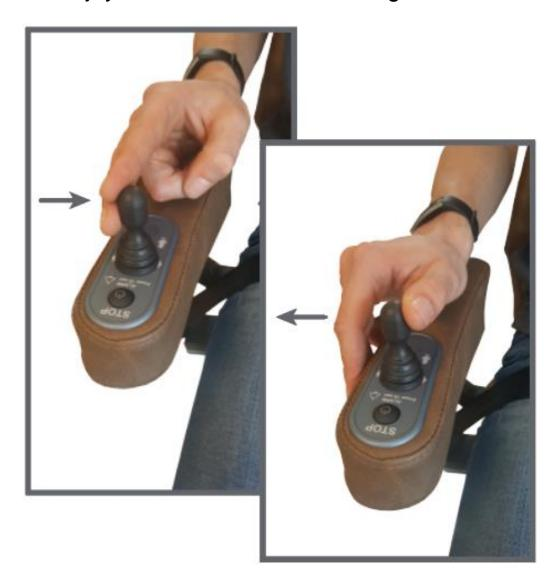
Swivel is a movement which will make standing up from the stairlift easier. The seat will be slightly turned compared to the carriage. At the end of the rail or at the charging point. Push the joystick one more time to turn the seat automatically.
